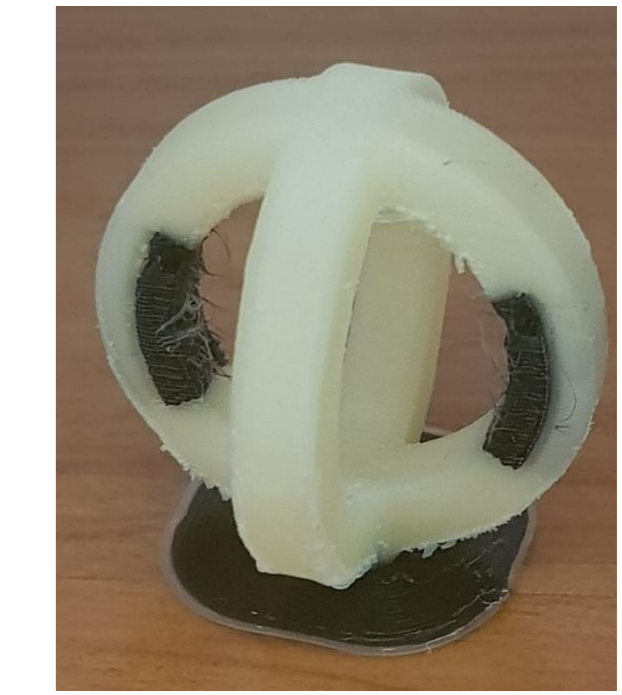
Figure 12 – Production of the double-ring structure.
