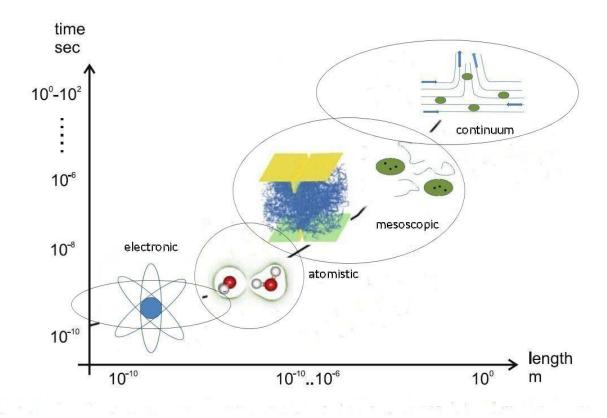
Fig 4 An illustration of entities in the different model types. (Pierre Severin, Coexpair and Olaf van der Sluis, Philips) The length and time scales to which the models can be applied are indicated by ellipses but as computers grow they are overlapping more and more. Hence the new classification!
