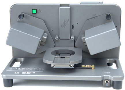
Alpha-SE (Woollam): Multi-wavelength 380-900nm, angles: 65°, 70°, 75° or 90° https://www.jawoollam.com/products
